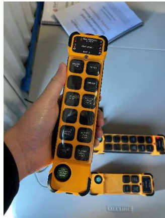
Local Wireless Controls w/ Wireless Re-charging
